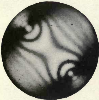
3.—Biaxial interference figure. Oblique position.
